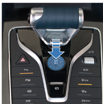
Turning off (Power meter "OFF" )
